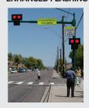
A pedestrian hybrid beacon is a beacon used to warn and control traffic and to assist pedestrians who are crossing a street or highway at a marked crosswalk. PUSH the BUTTON to activate the signal. Wait for the lights to flash and make sure cars and bicyclists see you and are stopping before you cross.
