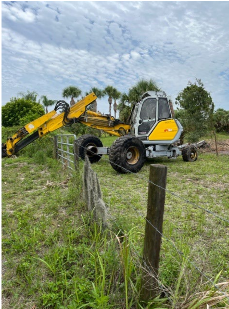
Photo of Menzi Muck, machine used to remove silt buildup within South Creek
